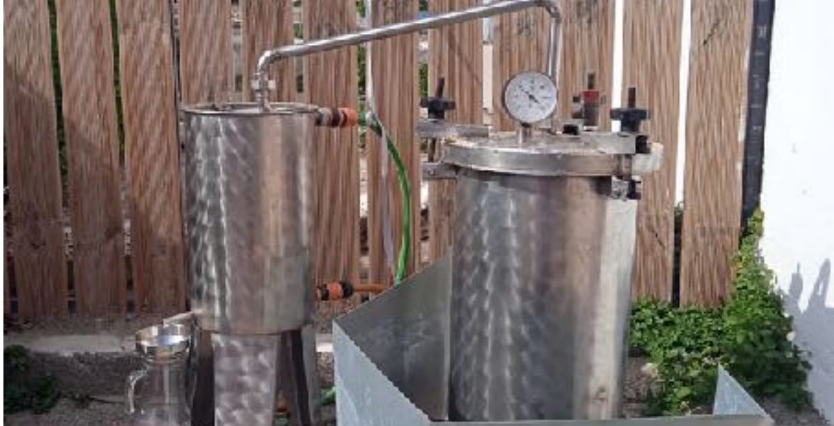
The still (right) and the cooler (left), with the glass carafe under the pipe in which we collect the hydrosol.
